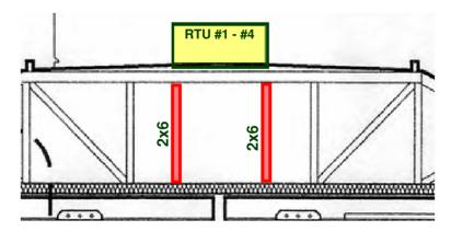
• RTU #5 - Install two vertical 2x6's below the RTU #5. Fasten the 2x6's, one on each side of each truss below the new RTU (six trusses minimum). Fasten each 2x6 to the side of the existing truss top and bottom chords with (5) 0.162" diameter X 3 ½". Angle the 2x6 from the edges of the new RTU down to the top of the CMU wall below. See sketch below:
