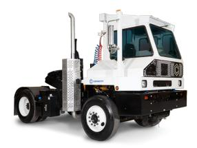
The TJ 9000 is a single-axle yard jockey truck with an impressive GCWR of up to 242,000-lbs. It can work anywhere: intermodal, warehouse and distribution, or for port trucking, and it handles rough surface conditions with ease.
