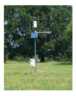
A typical tipping bucket raingage installation consists of a support pole buried in the ground, cabinet for instrumentation, tipping bucket, solar panel, and antenna.
