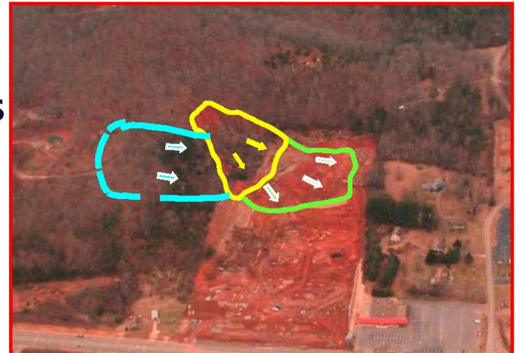
Landslide (weathered-rock slide)
